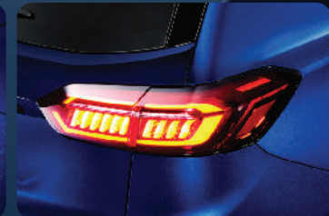
LED Rearlamp with Sequential Turn Signal
